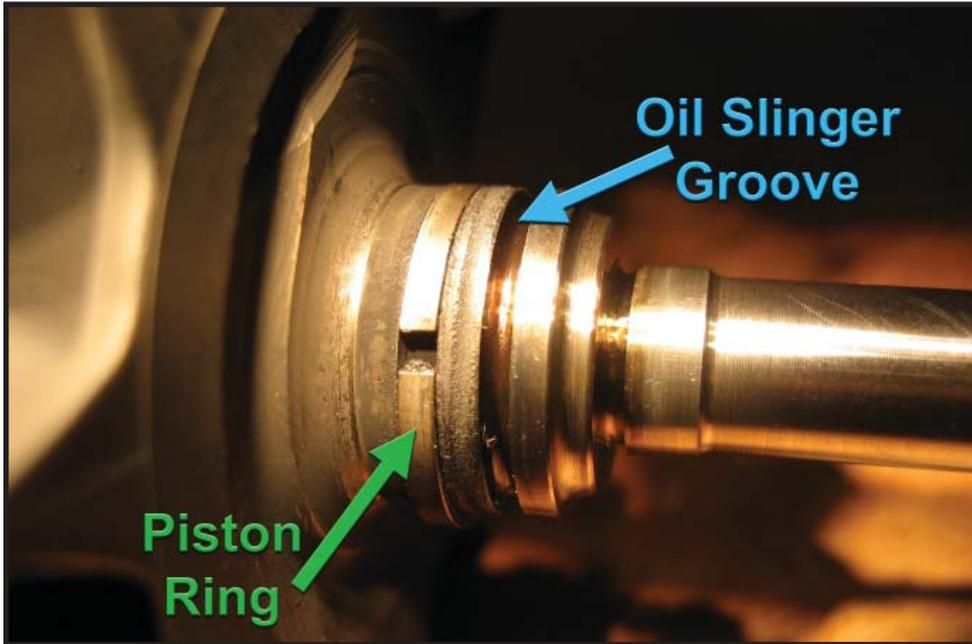
*Oil-sealing piston ring with gap visible, facing camera. Turbine wheel is at left, shaft is at right. These parts are used but in good condition – they have not been overheated and no coked oil is visible.*
