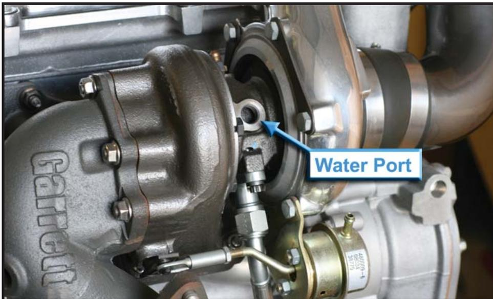
*Water ports are located on either side of the turbo’s center housing. Water should flow through the center housing from right to left, or left to right. If there are more than two ports to choose from, be sure to use one on either side of the center housing (don’t plumb both lines in on the same side).*
