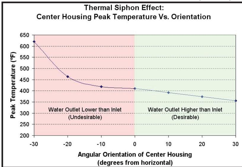
Graph showing center housing peak temperature vs. center housing orientation, as measured during heat soakback testing. Green zone to right shows lower temperatures resulting from proper water line setup, with outlet port higher than inlet. Red zone to left shows dramatic temperature increase as housing is rotated in the “wrong” direction, with the water outlet port lower than the inlet.
