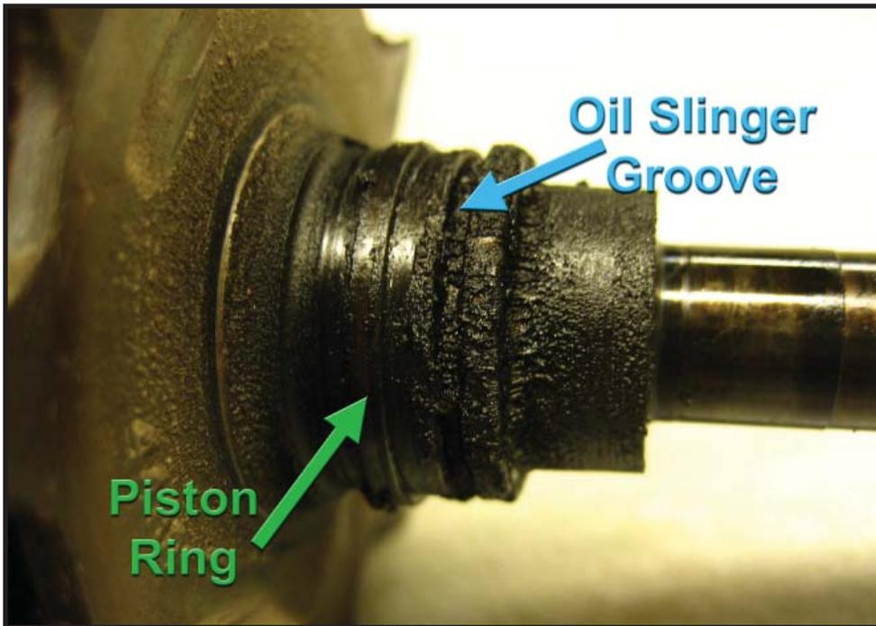
*Similar turbine wheel & shaft assembly, but this one has been repeatedly overheated. Piston ring groove and oil slinger groove both contain coke. If this piston ring has not yet collapsed, it is only a matter of time before it does. Severe bluing (discoloration) of the steel shaft on right is also visible, indicating the turbocharger has not been properly cooled or has operated above the maximum rated temperatures.*
