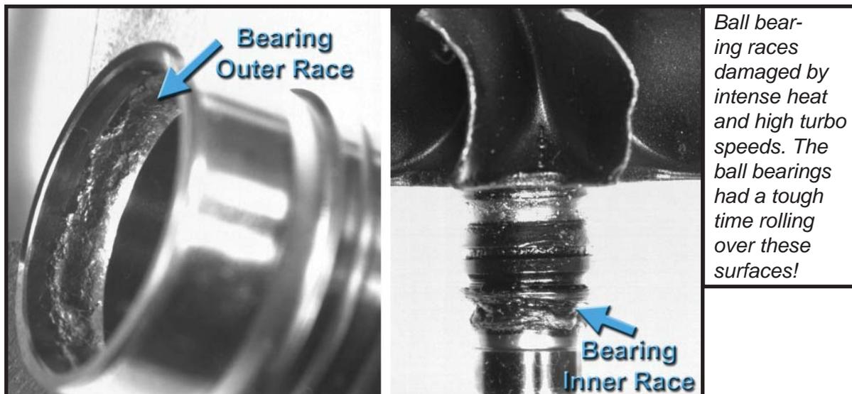
Each individual ball bearing inside the Garrett® dual ball bearing cartridge is held in place by a retainer, and there is one retainer per set of balls: one on the compressor side of the turbo and one on the turbine side. Elevated temperatures can also damage these retainers, which can lead to severe shaft motion (or play), wheels rubbing in housings, and again – catastrophic turbo failure. Keep your bearing retainers happy – don't over-cook them!
